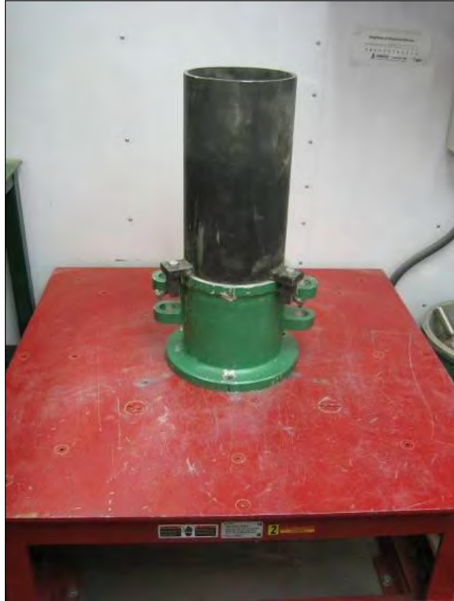
Figure 32. A 6-in. diameter mold on an electromagnetic vibratory table
