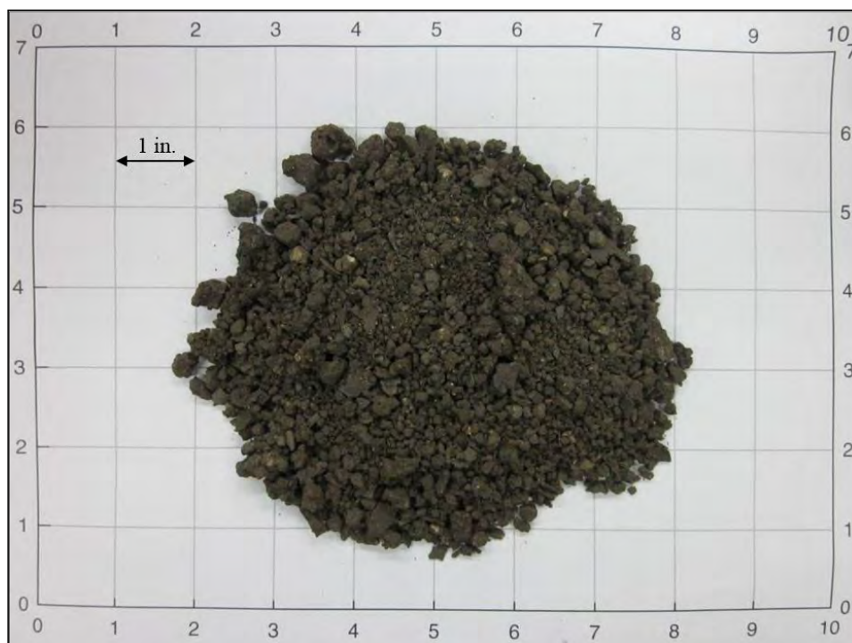
Figure 49. 2011 Texas fat clay at 15.5% moisture content
