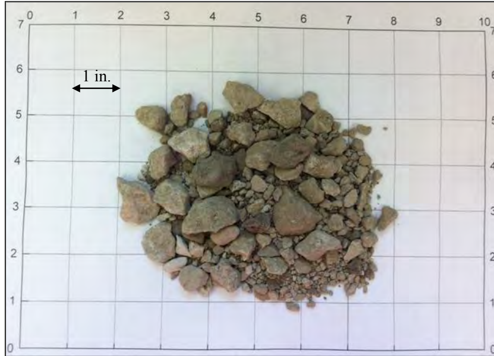
Figure 83. RPCC and RAP mixture (110°C oven-dried)
