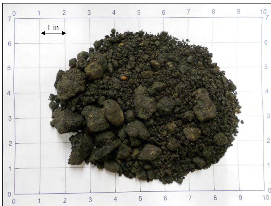
Figure 52. 2011 Manatt's RAP at 6.5% moisture content
