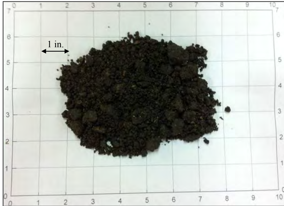
Figure 79. 2012 RAP at 4.8% moisture content
