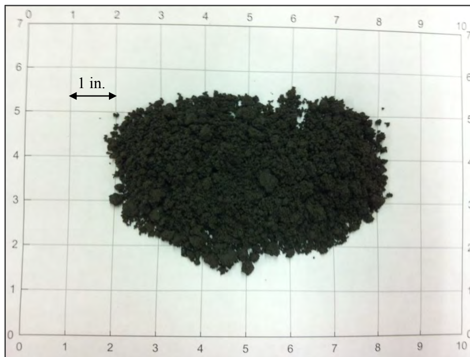
Figure 58. WCF fly ash at 23.0% moisture content
