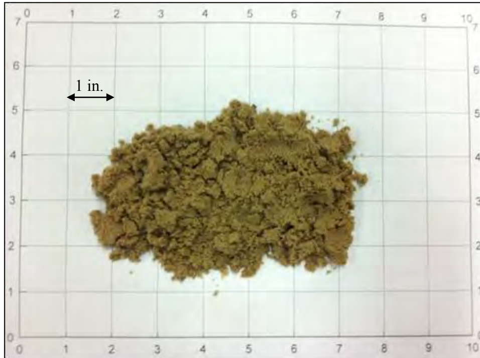
Figure 76. Florida highway 9B embankment fill at 7.1% moisture content
