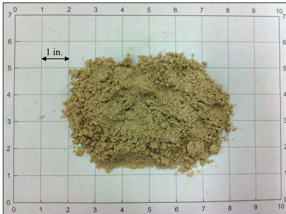
Figure 64. Temple gypsum at 9.4% moisture content
