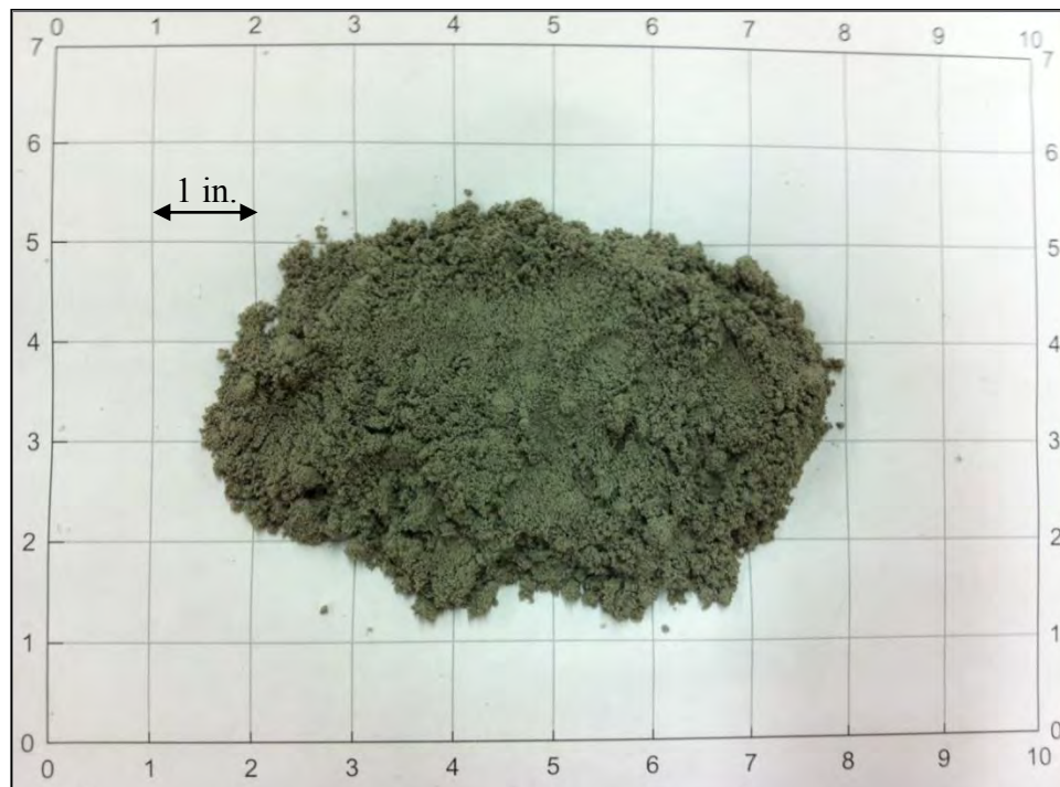
Figure 61. WCF gypsum at 16.0% moisture content
